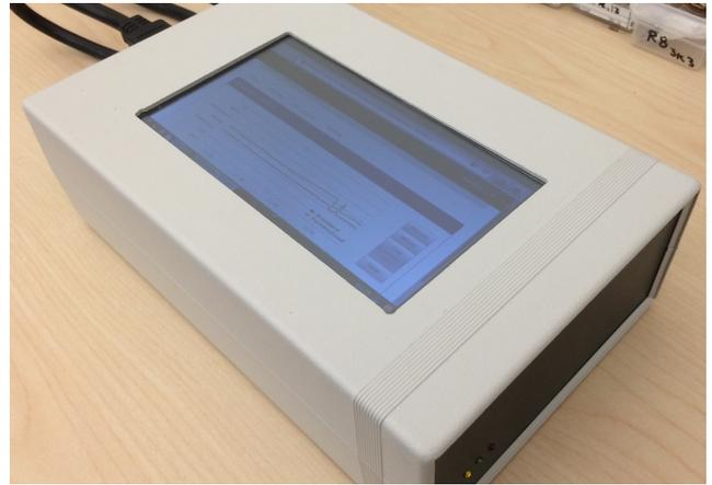
**Figure 5: For isolated installations of SPOT\*, a 7-inch touch screen LCD is mounted on the actuation box. This LCD is connected to the RPi inside the box and provides a local GUI to the user. In this configuration, which has the best privacy protection, occupancy data remains physically in the office.**
