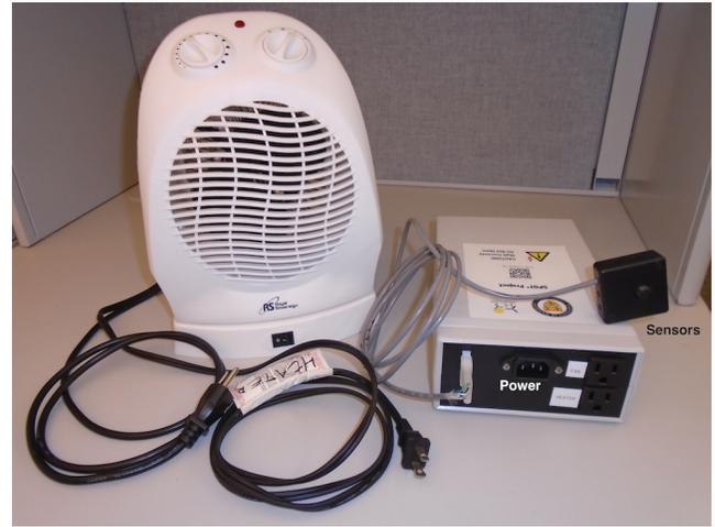
Figure 2: SPOT\* hardware. The fan/heater is shown on the left side, and the actuation box is on the right side, with the small black sensor placed on top. Two power cords of the modified fan/heater are connected to the box. In a typical deployment, the fan is placed on top of the box, and the desktop footprint is smaller than a single sheet of A4 paper.
