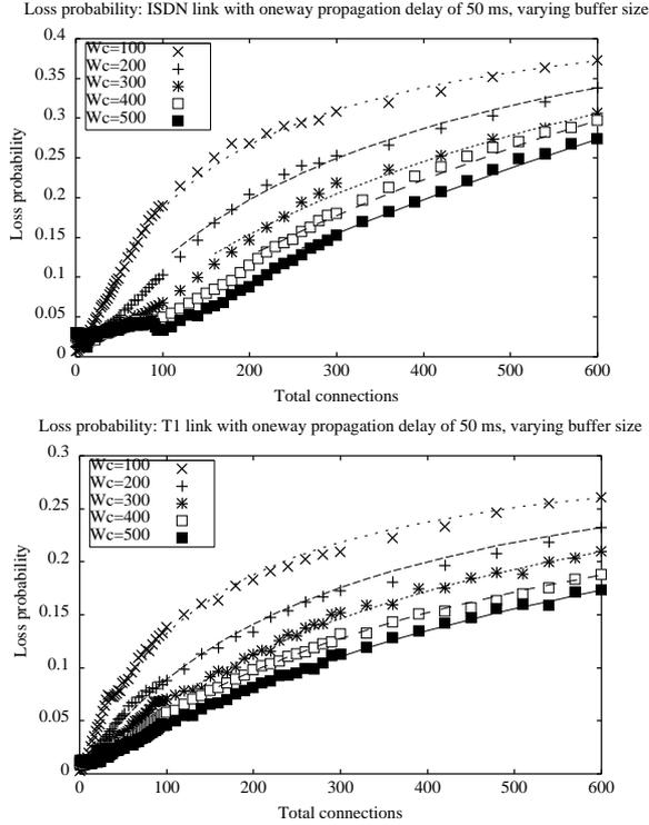
**Figure 10. Loss probability for a large number of connections: varying number of connections compete for the bottleneck link of either ISDN or T1. In both cases, propagation delay = 50 ms. The loss probability curves match very well with hyperbolic curves when the number of connections is large, where the parameters of the hyperbolic curves are given in Table 1.**
