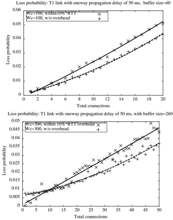
**Figure 17. Loss probability for a small number of connections** after adding random processing time of up to  $10\% \cdot RTT$  at TCP source: varying number of connections compete for the bottleneck link of T1 link with  $delay = 50\text{ ms}$ . The loss probability grows linearly when the number of connections is small.
