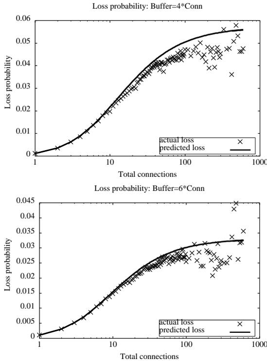
**Figure 3. Loss prediction for large pipe case: A varying number of connections share T1 link with one-way propagation delay of 50 ms, and the bottleneck buffer is either 4 times or 6 times the number of connections.**
