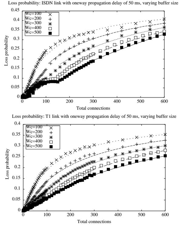
**Figure 18. Loss probability for large number of connections** after adding up to  $10\% \cdot RTT$  at TCP source: varying number of connections compete for the bottleneck link of either ISDN or T1. In both cases, the one-way propagation delay is 50 ms. The loss probability curves match very well with hyperbolic curves when the number of connections is large, where the parameters of the hyperbolic curves are given in Table 2.
