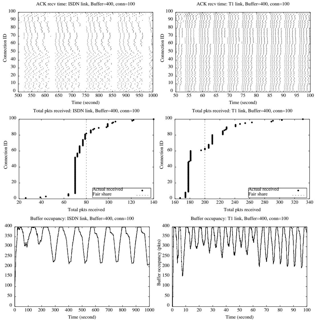
**Figure 2. Large pipe case leads to global synchronization: 100 connections sharing the bottleneck link of either ISDN or T1 with one-way propagation delay of 50 ms and bottleneck buffer size of 400 packets. Notice the buffer occupancy fluctuates from half to full periodically. Moreover there are periodic white stripes in the scatter plot of ACK arrival time, where during the white stripes all connections experience loss and try to recover them using fast retransmission.**
