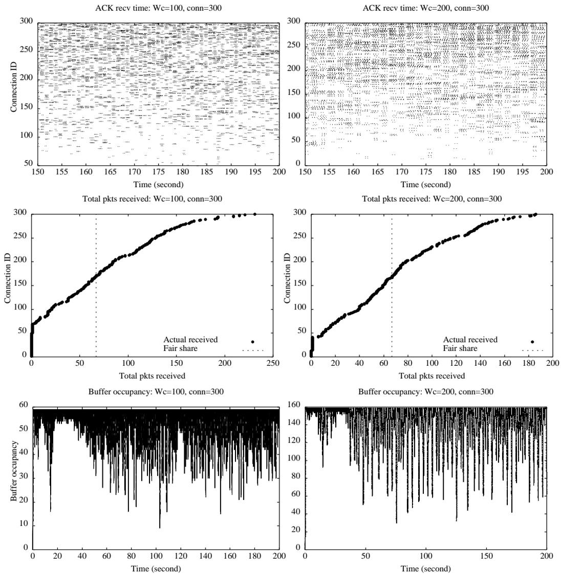
**Figure 4. Small pipe case: 300 concurrent connections compete for T1 link with one-way propagation delay of 50 ms and bottleneck buffer size of 60 (or 160) packets ( $W_c = W_{opt} + Buffer = 100$  or 200 packets). Note that the buffer occupancy fluctuates widely. Moreover part of connections receive little goodput as shown in the two graphs in the middle.**
