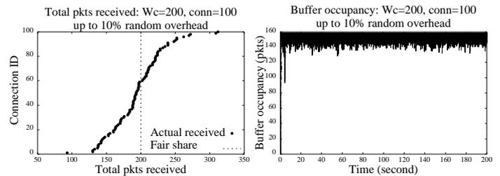
**Figure 14. Adding random processing time in medium pipe case: 100 concurrent connections compete for T1 link with  $delay = 50\text{ ms}$  and  $buffer = 160\text{ packets}$  ( $W_c = W_{opt} + Buffer = 200\text{ packets}$ ). The buffer occupancy is quite stable. In contrast to without random processing time, there is no local synchronization.**
