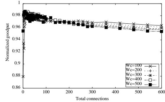
**Figure 15.** Throughput after adding random processing time of up to  $10\% * RTT$  at TCP source: varying number of connections compete for the bottleneck link of T1 link with propagation delay of either 200 ms or 50 ms.
