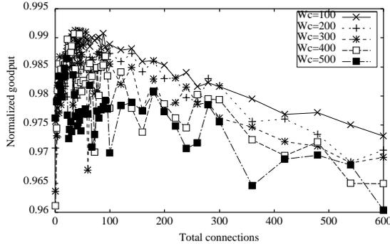
**Figure 8. Goodput: varying number of connections compete for the bottleneck link of either ISDN or T1. In both cases, delay = 50 ms.**
