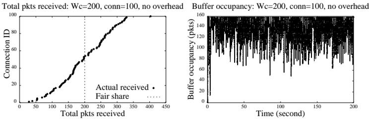
**Figure 6. Medium pipe case: 100 concurrent connections compete for T1 link with  $delay = 50 ms$  and buffer = 160 packets ( $W_c = W_{opt} + Buffer = 200$  packets). Buffer occupancy fluctuates widely, and there is local synchronization within some groups.**
