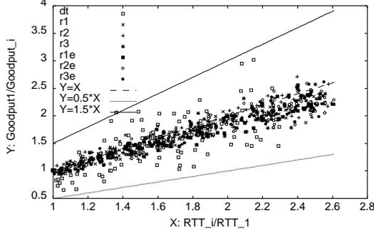
Figure 35. Comparison between the effect of RED gateway and the dropping tail gateway on 8 TCP flows with all different RTT's.
