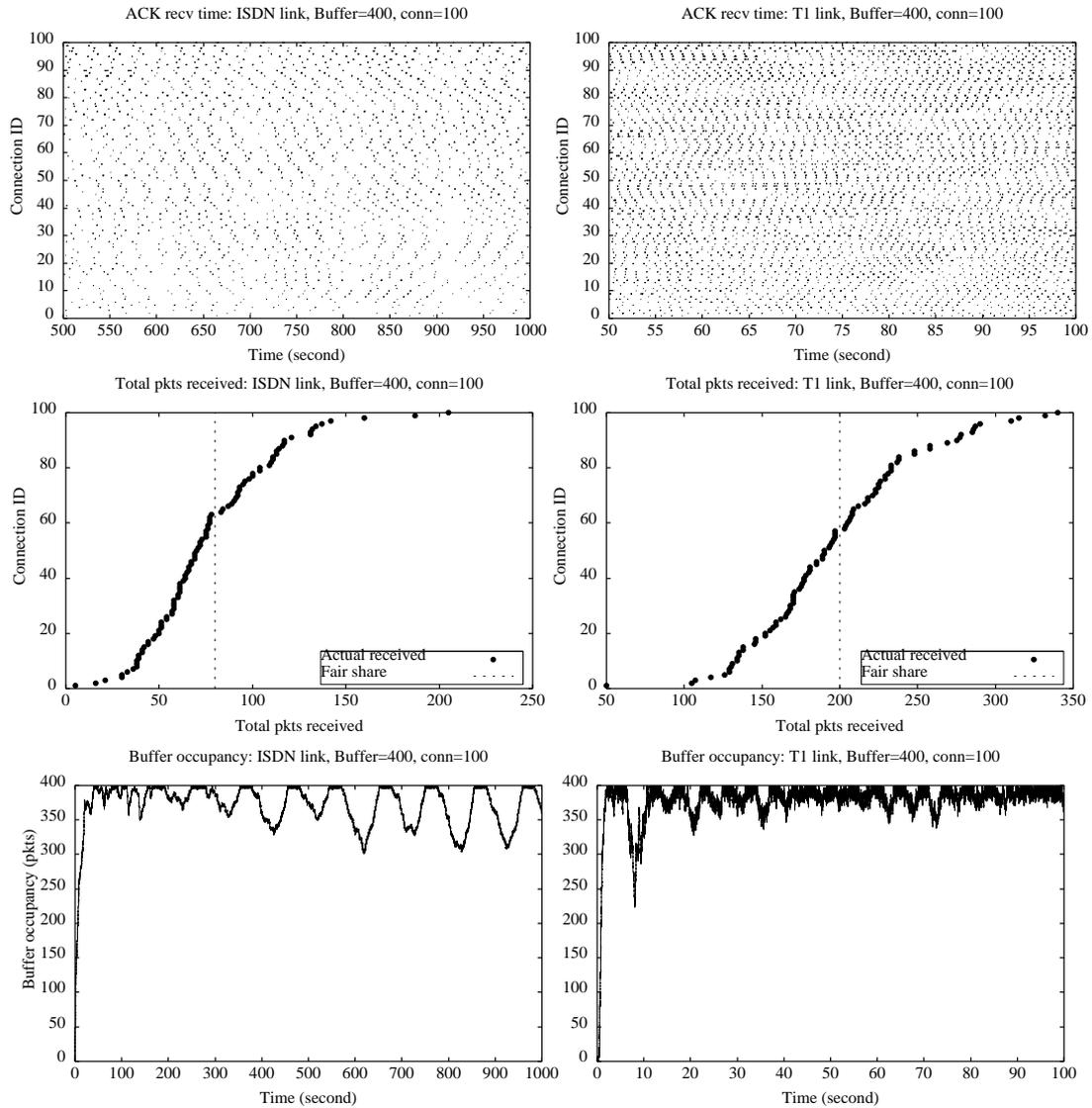
**Figure 11. Adding random process time in large pipe case breaks down the global synchronization: 100 connections share the bottleneck link of either ISDN or T1 with one-way propagation delay of 50 ms and bottleneck buffer size of 400 packets. Compared to the case of without random processing time, the buffer occupancy is quite stable. Furthermore global synchronization disappears as shown in the scatter plot for ACK arrival.**
