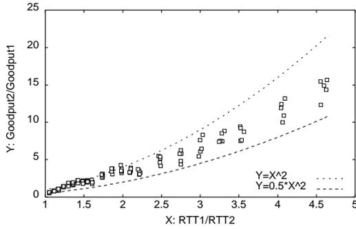
Figure 32. The effect of Drop-Tail queue ( $\delta t$  in Table 3) on 6 FTP sessions with 2 different RTT's. The bottleneck link has T1 capacity and 50 msec one-way propagation delay.  $PD_1$  varies while  $PD_2$  is kept at 102 msec.
