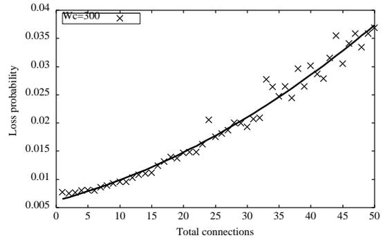
**Figure 9. Loss probability for a small number of connections: varying number of connections compete for the bottleneck link of T1 with delay = 50 ms. The loss probability grows quadratically when the number of connections is small.**
