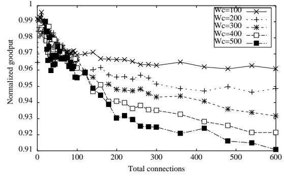
Normalized throughput: T1 link with oneway propagation delay of 50 ms, varying buffer size
